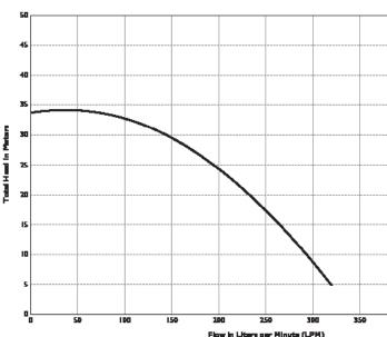
Note: Performance based on pumping solvent (0.78 specific gravity). Pressure is taken at the manifold discharge outlet. Fixed Speed 2.00 HP was powered by Three-Phase, 50 Hz, 415 Volt incoming supply.
