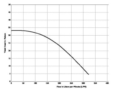
Note: Performance based on pumping solvent (0.78 specific gravity).
